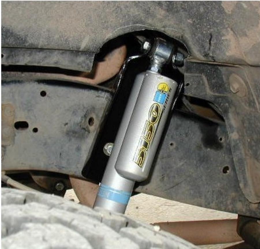
1st step is to remove the sheet steel half of the factory mount that's riveted to the frame with 2 rivets. You can grind the rivet heads off, use an air chisel, drill them out or even other techniques will work.
