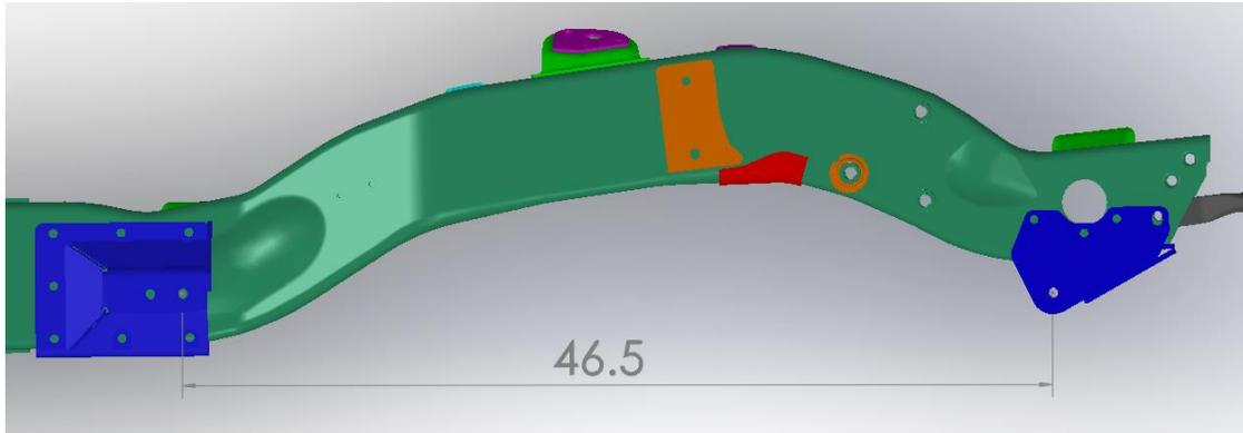
7. Mark the 9 mounting holes, drill them out and install the 7/16" hardware to mount bracket. Torque nuts to 38 ft. lbs.
