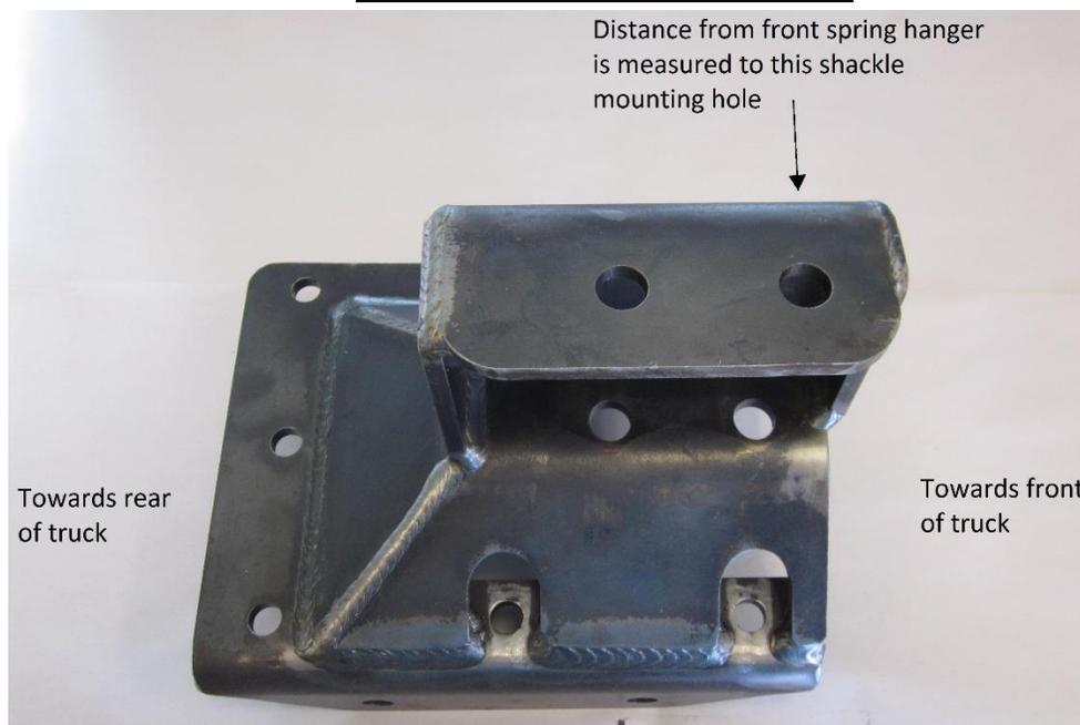
Position rear hanger such that the distance from the front spring eye bolt centerline to the **forward-most** upper shackle bolt centerline is 46-1/2". See drawing:
