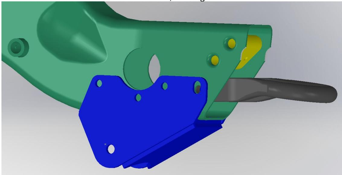
1. Remove the two bolts from the sides of the tow hooks on the front of the frame.
