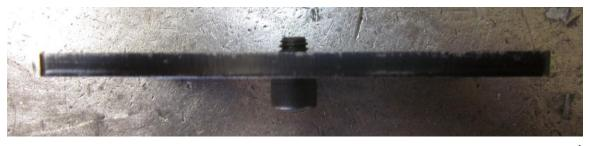
2. Cut off the exposed threads and grind it flush, a flap wheel works well.
