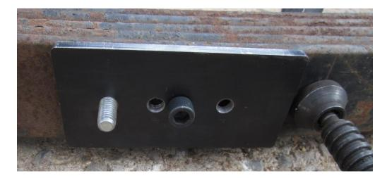
7. Cut off the exposed threads and grind it flush, a flap wheel works well.
