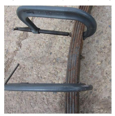
4. Remove the old center pin. A set of locking pliers on the round side of the bolt are often helpful.
