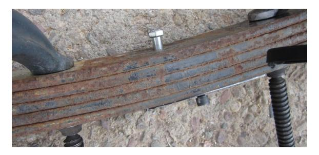
6. Thread 3/8" hex bolt into offset plate using the threaded hole with the corresponding offset you want to use. The plate is engraved with the different options. Snug is fine here, there isn't any force on these bolts, they just hold the spring pack together.
