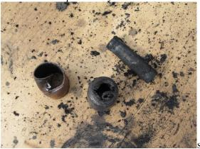
Once the rubber bushing assembly is out of the spring and shackle eyes you should be ready to put our bushings in. You will install two bushings halves, one sleeve and one greasable bolt into each spring eye:
