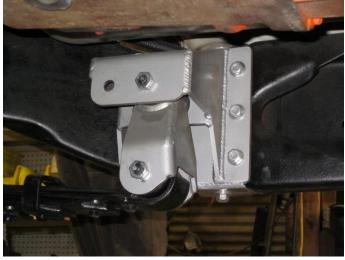
Mark all of the holes using the bracket as a template. Drill the holes with a  $\frac{1}{2}$ " drill bit.
