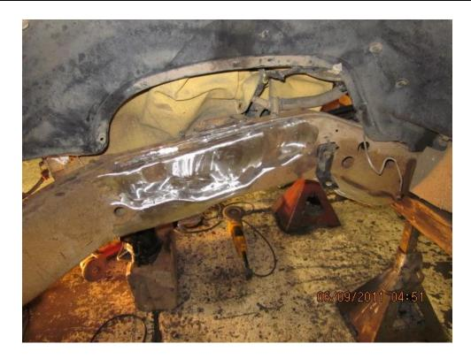
Install front hangers, additional holes will need to be drilled on the inside of each frame rail.  $\frac{1}{2}$ " x 1-1/2" bolts go in the outside of the frame rail to account for the bumper bracket,  $\frac{1}{2}$ " x 1-1/4" bolts go on the inside and 7/16" x 1-1/4" bolts go in the bottom.
