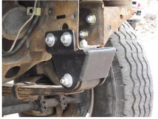
Position rear hanger such that the distance from the main eye centerline to the upper shackle bolt is 46.5". You will be using the forward most shackle bolt location, the bent piece of the bracket goes towards the front of the truck.
