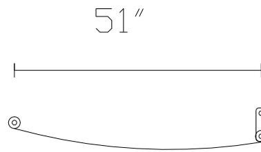
This is the passenger's side rear shackle hanger bracket, the notched and bent piece goes towards the front of the truck:
