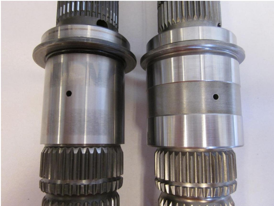
The depth on the pump seal is important. This seal below has been driven beyond flush and can cause problems:
