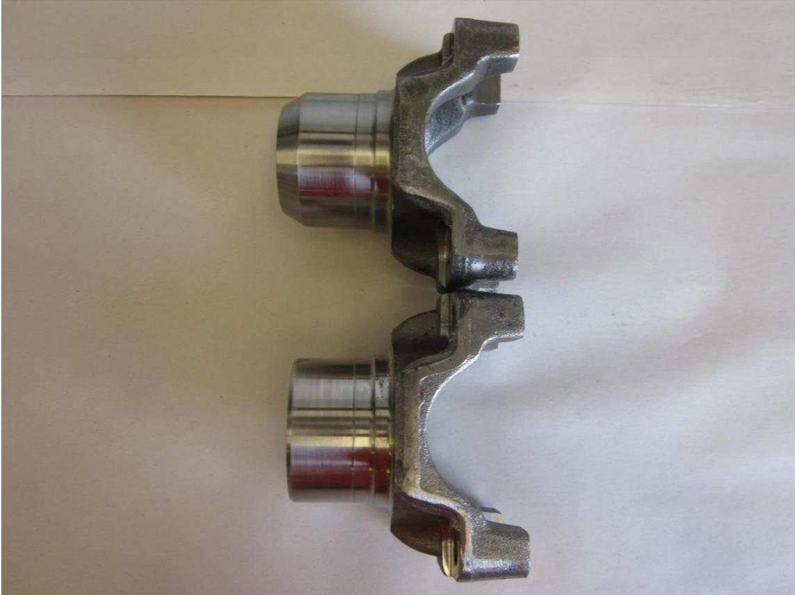
Most 32 spline yokes will need to be shortened by about ¼”, the length of the spline in the yoke needs to be 1-11/16”.
