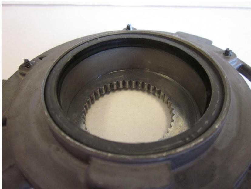
This seal has been driven exactly flush, this is correct. Regardless of how your seal was when you took it apart, make sure the seal is flush with the pump housing when you reassemble it.
