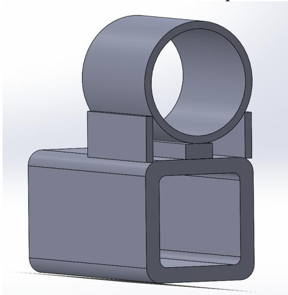
9. Double check that the traction bar and frame crossmember line up the way you want them to, remove traction bar from brackets and finish weld the bracket to the axle tubes.
