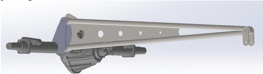
7. Tack weld the axle side bracket into place.
