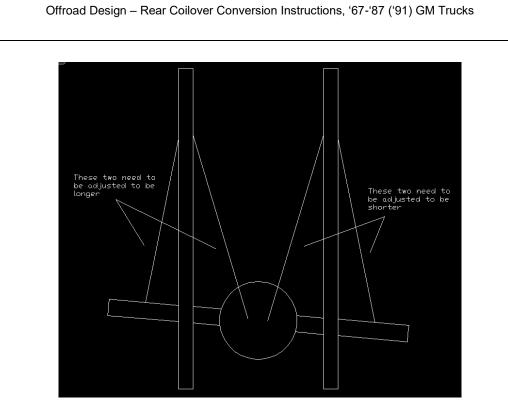
By adjusting the link length as shown above, you can make the axle square with the chassis:
