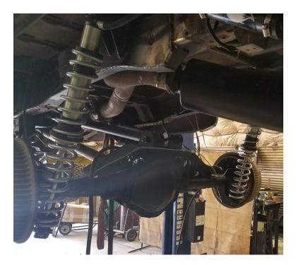
15. With the springs removed from the shocks, mount them to the frame and axle. Everything should be ONLY tack welded at this point.
