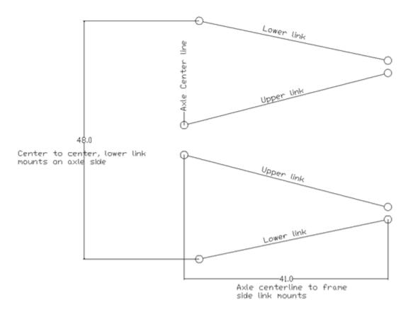
This is a side view and here again, most everything is set by our brackets. The main point here is to make sure the bolt hole for the lower link mount on the axle side is 1" above axle centerline with your pinion angle within a couple degrees of its final rotation.
