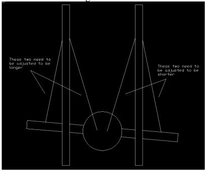
By adjusting the link length as shown above, you can make the axle square with the chassis:
