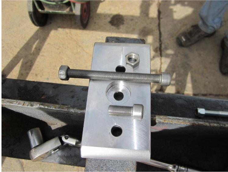
2. Run the center pin through the hole in the center of the new U8003 leaf and tighten the nut in the cutout in the top of the leaf. The center pin end must be below the top surface of the zero rate.
