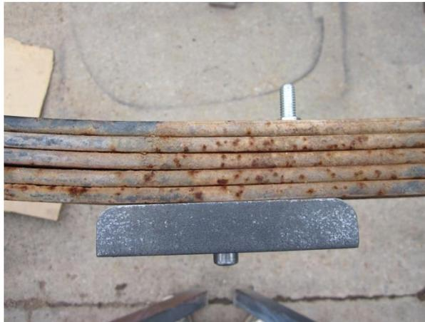
4. You will need to drill a clearance hole in your upper ubolt plate for the nut on top of the spring. Measure 1" or 1.5" off center of the ubolt plate and drill the hole. It needs to be about 3/4" in diameter. Now you're ready to re-install the axle.
