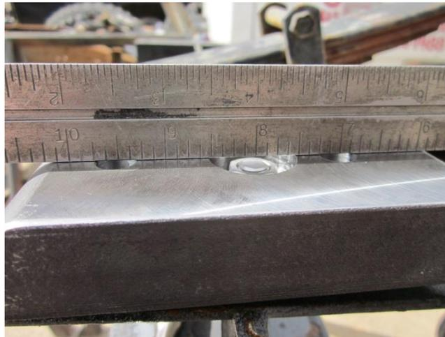
3. Install the supplied 3/8" x 3 1/2" bolt with the head on the bottom of the new leaf through one of the offset holes. To move the axle forward, the leaf must be offset toward the front of the truck. Pick the hole in the leaf that moves the axle the amount you want, one hole is 1", the other is 1.5" offset. Make sure you use the same hole on both sides of the vehicle! Run the 3/8" bolt through the hole in the
